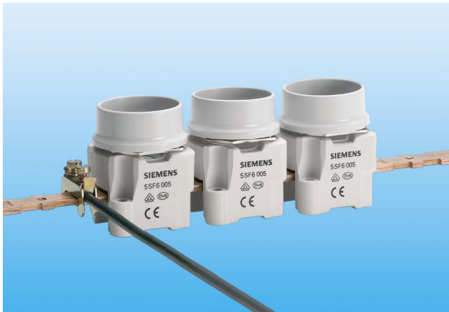
5SF6 005 DIAZED bus-mounting base DII for 25 A with terminal version "B" mounted onto an EZR 5SH3 500 busbar. The feeding conductors are clamped to the 8JH4 122 bus-mounting terminal. The busbar has a load capacity of up to 150 A.
