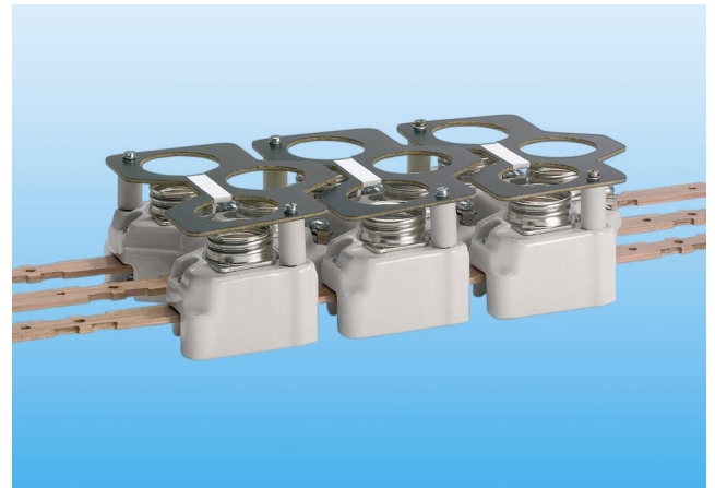
3-phase 5SF2 07 DIAZED bus-mounting base DII for 3 x 25 A with terminal version "B" mounted onto an EZR busbar. The busbar has a load capacity of up to 150 A.
